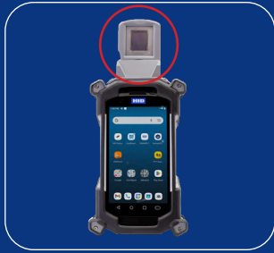
HID NOMAD FAP 30 fingerprint reader on swivel mechanism that can be stowed when not in use.
